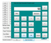
You can either directly enter a percentage by pressing on the Tensile correction button and enter on the popup keypad or press Auto Correction, enter the desired angle as prompted and then resulted angle. It automatically enters a tensile correction. When a job is saved, it saves the tensile correction for that job.
